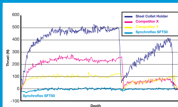
Graph illustrates the final hole tapped by each tap driver.
